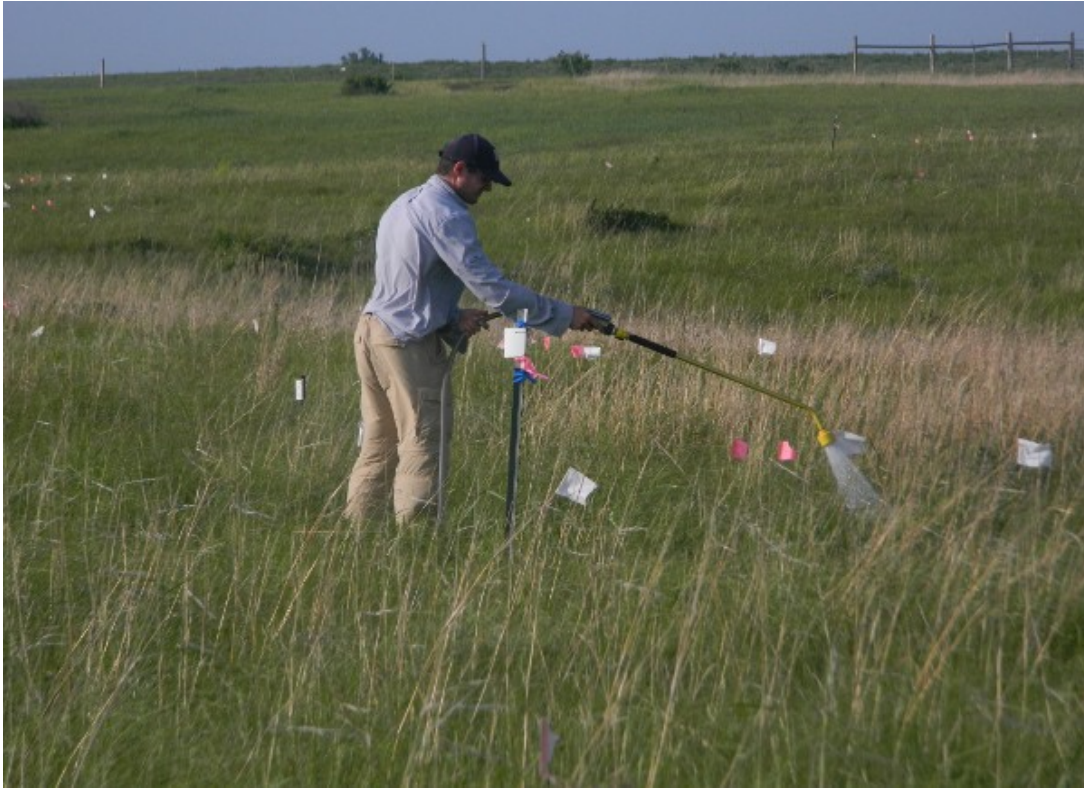
Figure 2: Water addition in the 4B watershed at KPBS via hand-held wand and flow meter in a wet treatment plot in late June. Water was applied weekly to these plots so that they received 130% (~800 mm) of the growing season mean rainfall and stayed consistently wet. Water application began in June 1 and continued through August 31, 2013.
