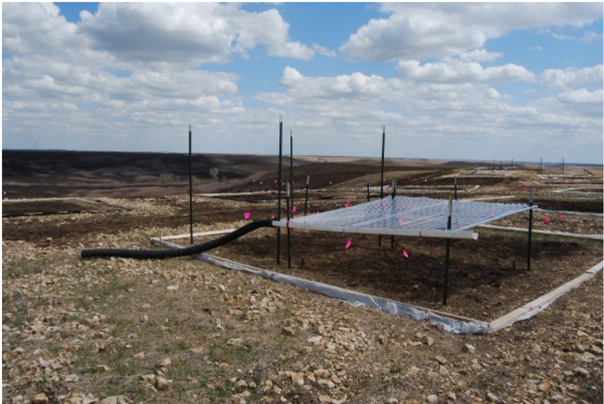
Figure 1. A rainout structure just after it was installed in April, 2013 on the recently burned 4B watershed at KPBS. The roof was constructed with clear, polycarbonate plastic and was 2.5 x 2.5 m. A drainage tube collected runoff from the roof and shunted it out of the plot. The plot was trenched to 0.5 m and a plastic liner was installed to prevent belowground infiltration from outside of the plot. Late spring drought roofs were in place April 20 – June 22 , early summer drought roofs were in place May 22 – July 2, and mid-summer drought roofs were in place June 22 – July 26. The goal of each drought treatment was to exclude ~ 150 mm of precipitation.
